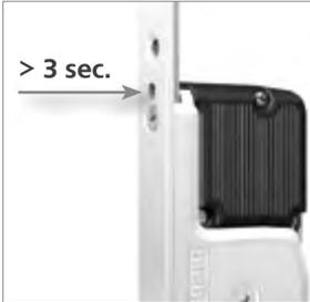
1. Carefully press the programming button on the Smart radio module for at least 3 seconds.
