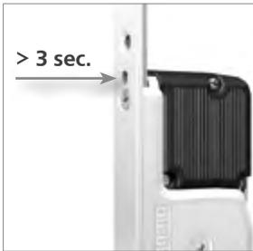
1. Carefully press the programming button on the Smart radio module for at least 3 seconds.
